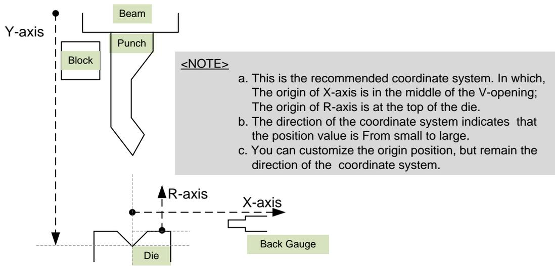
Figure 3-10 The direction of servo-axes
