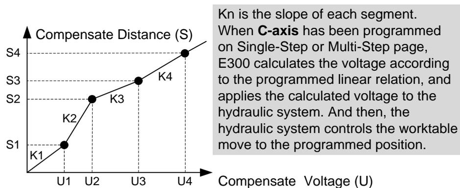
Figure 3-14 Linear relation between **Compensate Distance** and **Compensate Voltage**
