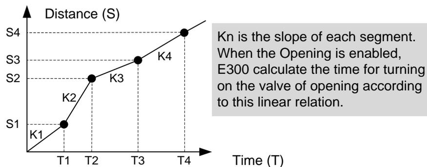
Figure 3-18 Linear relation between **Distance** and **Time**
