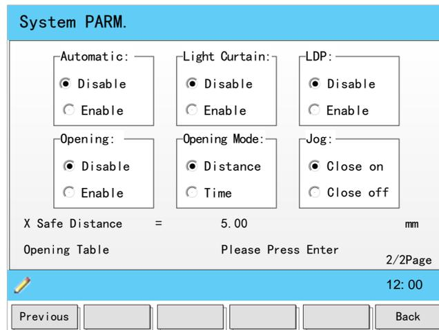
Figure 3-16 Page 2 of System parameters (2/2)
