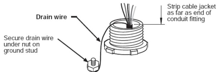
Figure 2-2 Connecting Shield Drain Wire to Ground
