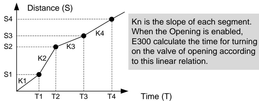
Figure 5-1 Linear relation between **Distance** and **Time**
