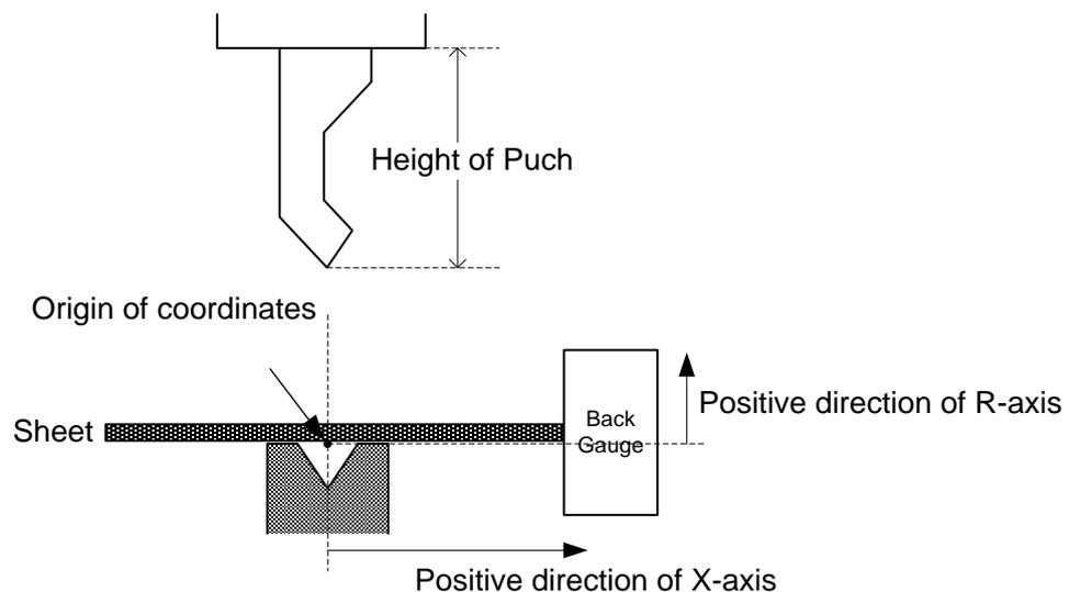
Figure 3-21 Coordinate system of machine
