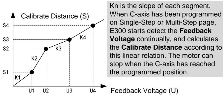
Figure 3-12 Linear relation between **Calibrate Distance** and **Feedback Voltage**
