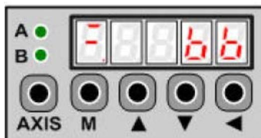
Figure B-1 The operation panel of the EDS
